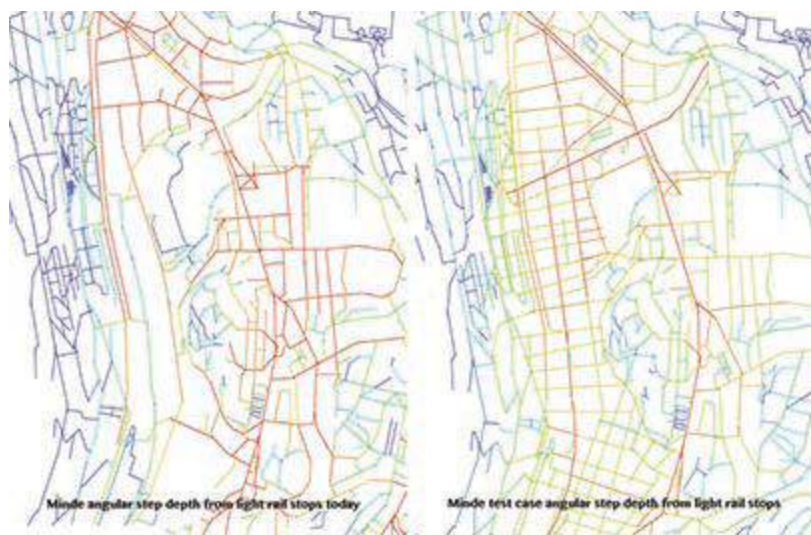
Figure 7 – Angular step depth from light rail stops showing changes in public transport accessibility with Mindemyren as a test case
