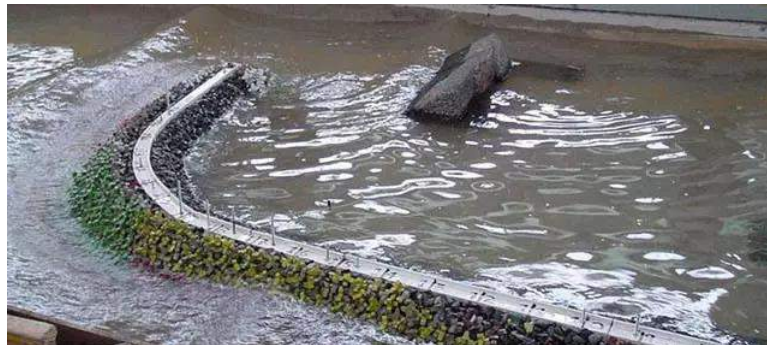
Figure 4 - Establishment of Physical Hydraulic Model
