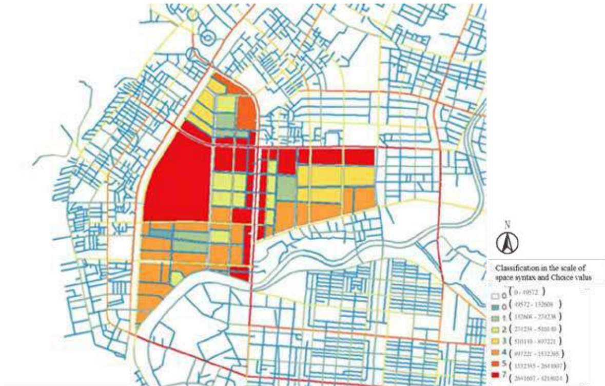
Figure 19 The result of Space Syntax by calculating the value of choice at the scale of blocks
