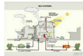
21. BedZED technical section showing building physics
