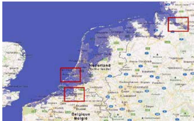
3. Flooded land if sea level rises only 1 meter and no precautions are taken .
